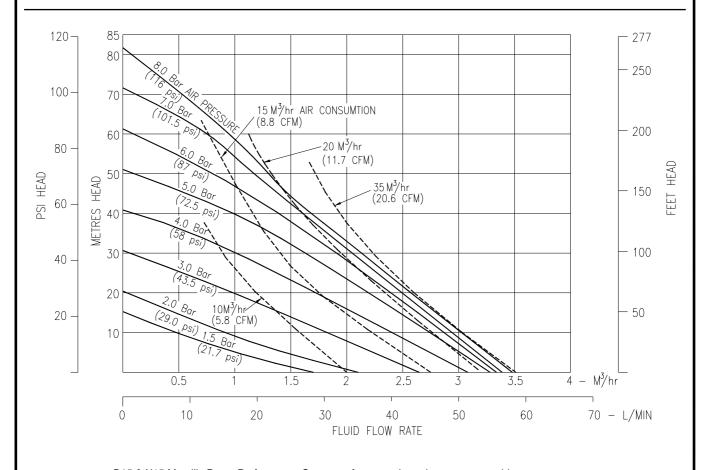
B15 & X15 Metallic Pump Performance Curve, performance based on water at ambient temperature
