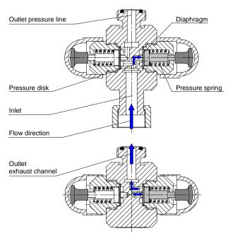
If the admission pressure increases beyond the opening pressure, the diaphragm is raised against the spring force and the valve opens.
